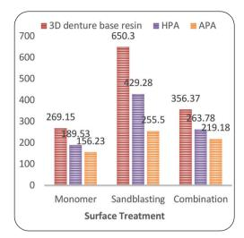
Fig. (6) Column chart showing flexure strength mean values for Different types of surface treatment of repairing materials
