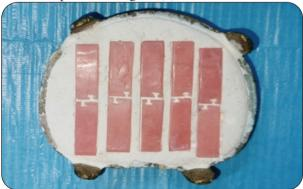
Fig. (3) Flasking the sectioned specimens
