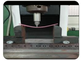
Fig. (4) Flexural strength Test Setup
